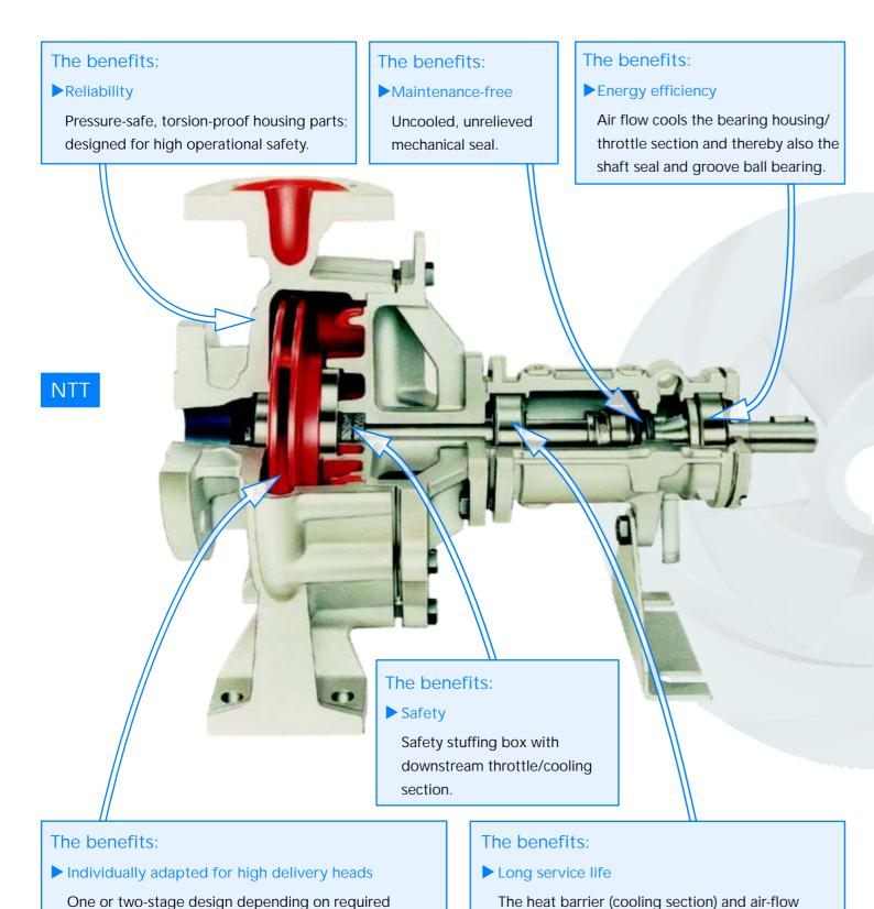
The NTT, NBT and NIT product series are ideal for moving mineral-based thermal oils. Their mechanical seals are located behind a heat barrier, where they are protected from high temperatures. The result is that simple standard gaskets (antimony-carbon/SiC) have a very long service life when used in the pumps. All three types are also available as two-stage versions with the same external dimensions, making them ideal for small flow rates with high delivery head.
